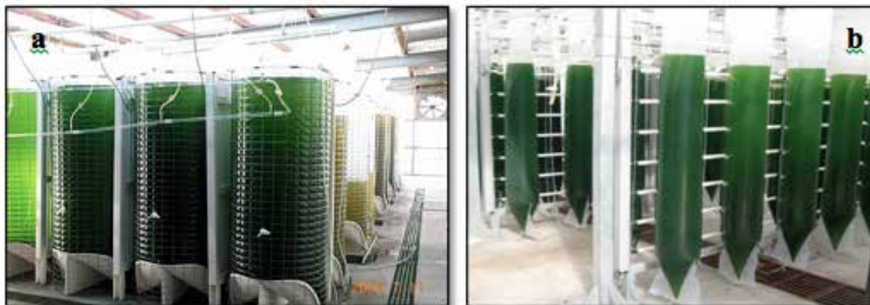
Figure 7. the stand-up pouch or the punching bag systems of photobioreactors.
