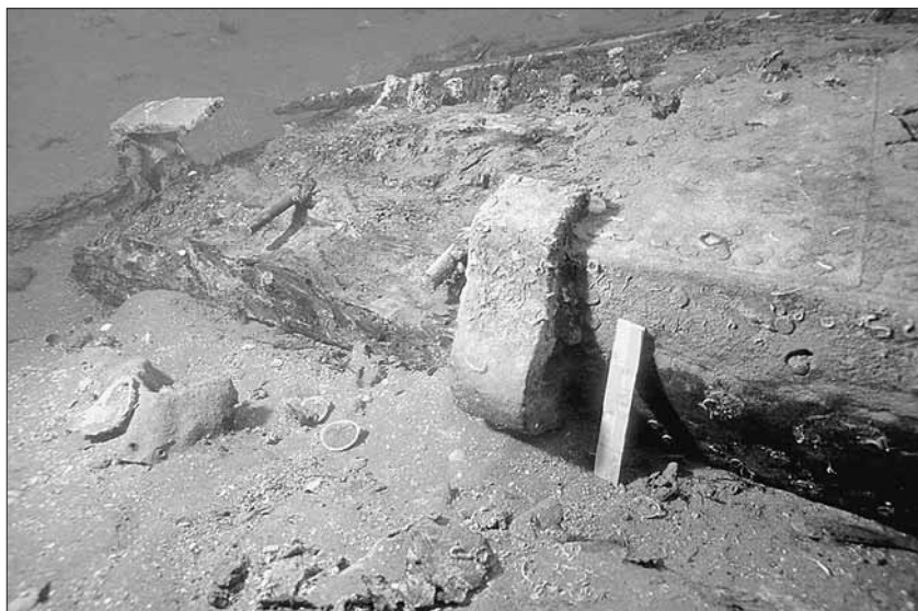
Fig. 6 Mercure . – The gudgeons on the sternpost (Photo S. Caressa).
