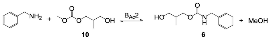
Scheme 5 Formation of 3-hydroxy-2-methylpropyl N -benzyl carbamate 6 .
