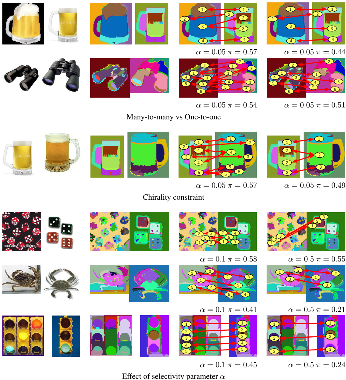
Figure 1. Region matching: the first four columns show the original images and the extracted segments, while columns five to eight show the resulting matches. The first two rows show the result of enforcing one-to-one correspondence, the third row show the result of enforcing chirality (handedness) of the matching segments, while the last three rows show the effect of changes in the selectivity parameter \alpha .
