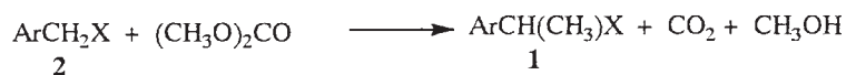
Scheme 8. Mechanism of the mono- C -methylation of CH 2 -active compounds (X = CN, CO 2 CH 3 ) with DMC.
