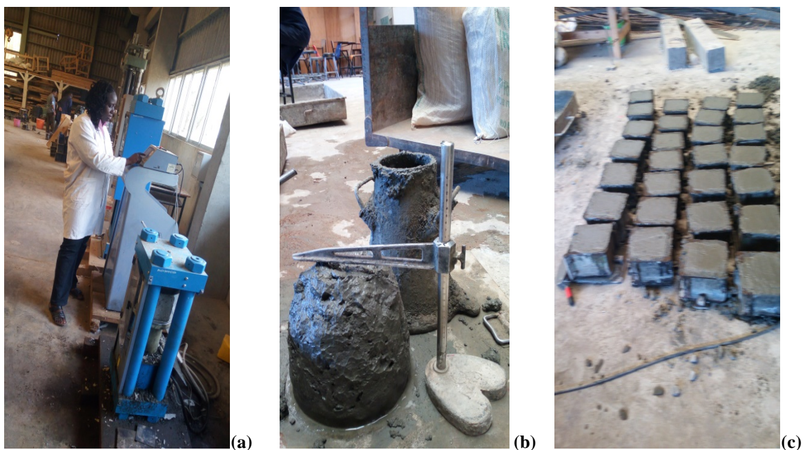
Figure 1: (a) Compressive strength testing machine, (b) slump test cones and (c) casted concrete cubes
