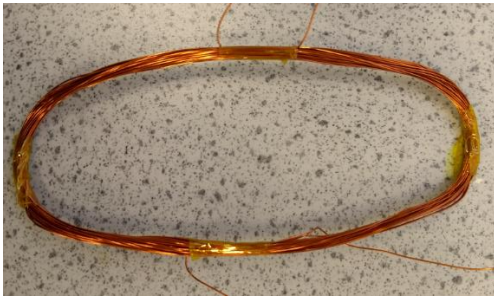
Fig. 3. Unaged coil employed for the investigation.
