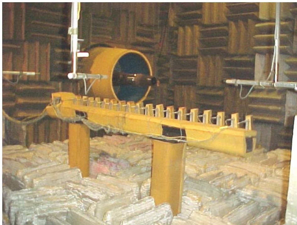
Figure 3. Acoustic Research Tunnel showing model scale nozzle as viewed from aft microphone angle.
