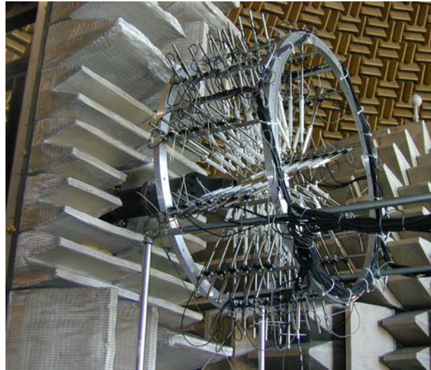
Figure 4. 78 microphone array tested in NASA GRC SHJAR for subsonic jets.
