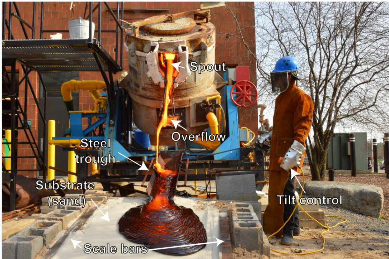
Figure 5. High-volume, gas-fired tilt furnace used for melting batches of basaltic- to basaltic-andesite lava at the Syracuse University Lava Project.
