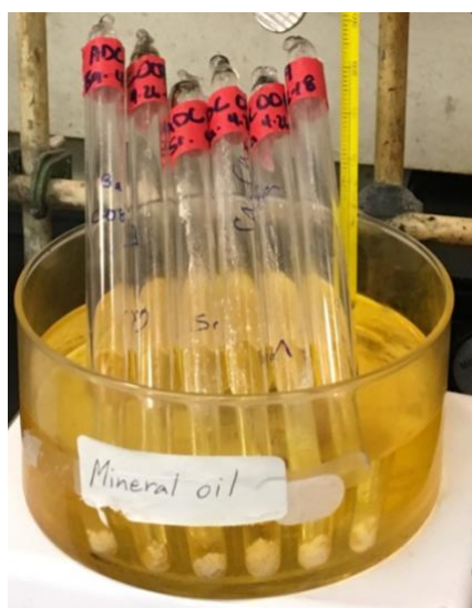
Figure 3.2 Reactions in Carius tubes monitored at various temperatures to induce crystallization.
