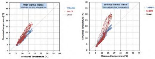
Figure 3. Simulated vs Measured surface temperatures of the substrate for models with and without thermal mass.
