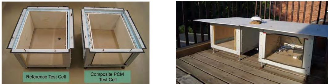
Figure 2. Experimental test cells: the test cell on the right contains the investigated PCM system.
