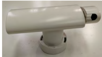
Figure 1 The IR scanning device of the Comfort Eye
