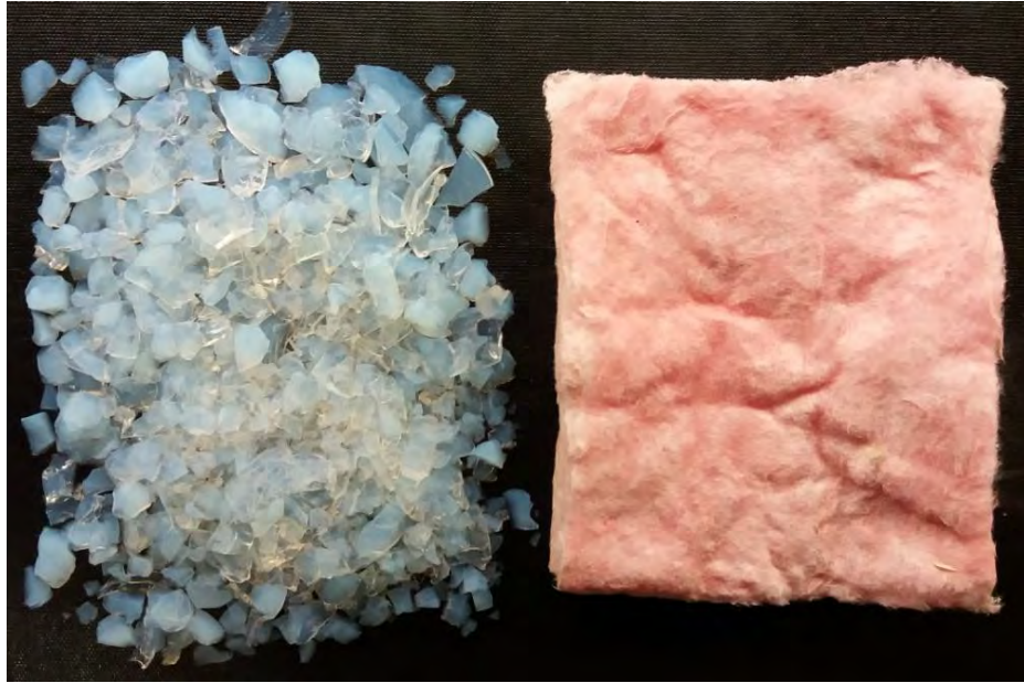
Figure 4. Authors' produced aerogel granules (left) and aerogel-enhanced blankets obtained embedding a fiberglass panel with precursor aerogel before the drying process (right).
