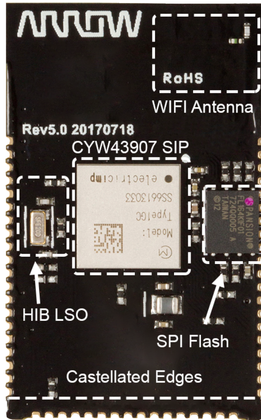
Figure 7: An annotated image of the Quicksilver module.
