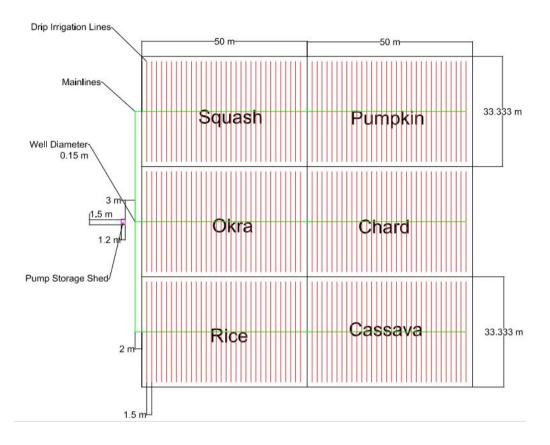
Figure 4: Altered drip irrigation map layout of the 100 meter by 100 meter field.
