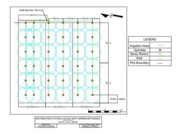
Figure 5: Initial sprinkler map layout of the 100 meter by 100 meter field as well as the sprinkler radii.
