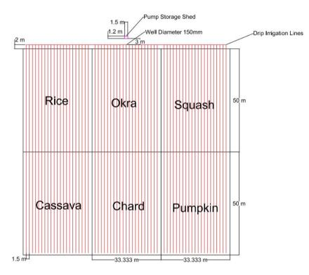
Figure 3: Initial drip irrigation map layout of the 100 meter by 100 meter field.
