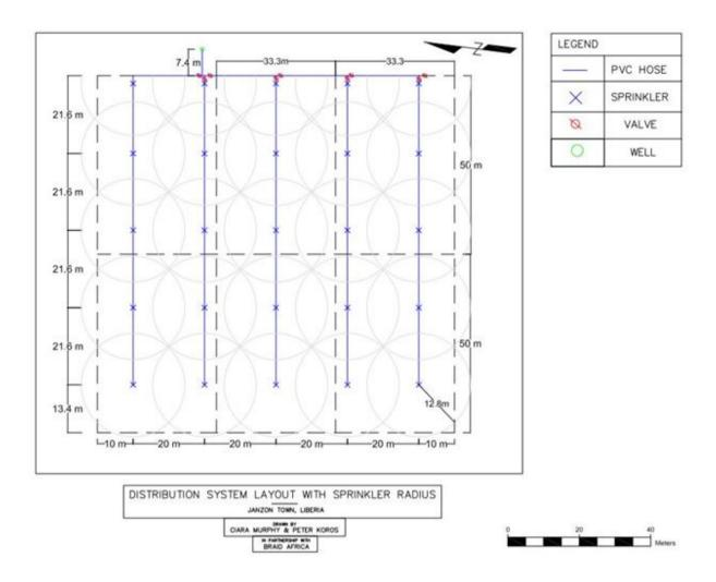
Figure 6: Updated sprinkler map layout of the 100 m by 100 m field with sprinkler radii.
