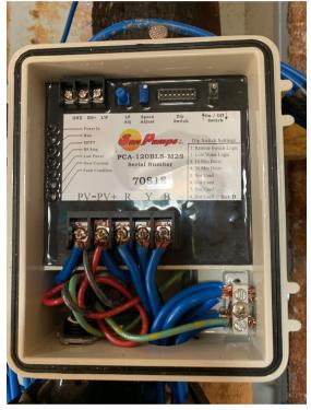
Figure 10: The wiring that connected the solar panels and pump, and the controls of the pump's flow rate.
