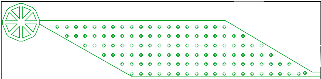
Figure 6. AutoCAD design of micropillar array within microfluidic microinjection chip. Micropillars are utilized to (1) redistribute entering worms and prevent animal clustering, and (2) filter debris to prevent clogging of upcoming narrow flow channels.
