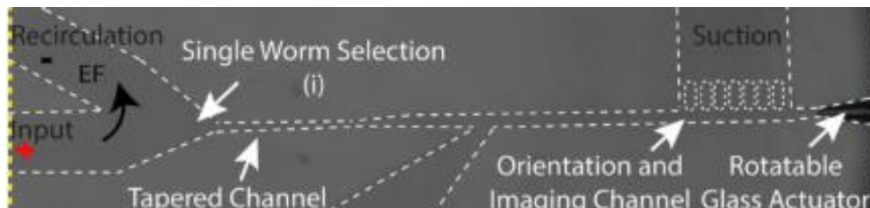
Figure 2. Schematic representation of a microfluidic chip that uses a glass actuator to rotate a single worm 7 .
