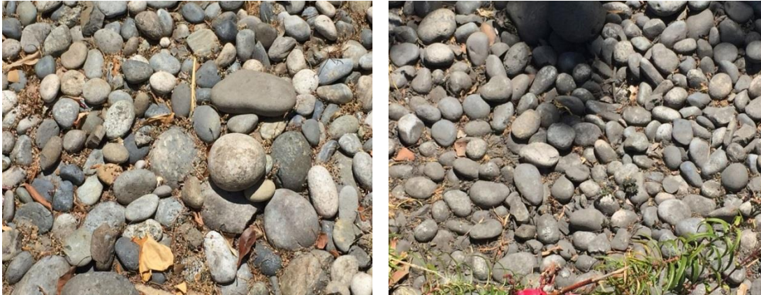
Figure 8. Municipal Site 14 on the left (Infiltration Rate: 27.5 in/hr.) and Municipal Site 15 on the right (Infiltration Rate: 15.2 in/hr.) (Photo by author).
