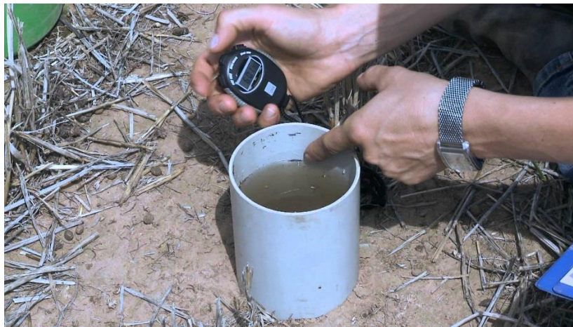
Figure 5. Basic infiltration test (Catchment Management Authority, 2012).
