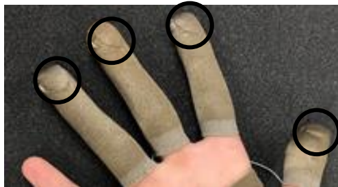
Figure 2.1 – Capacitive sensors are located at the fingertips (volar pad) of the thumb and first three fingers.
