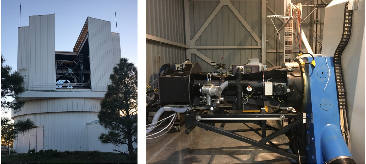
Figure 1.6 The Astrophysical Research Consortiums 3.5 meter telescope and enclosure (left) located at the Apache Point Observatory in Sunspot, New Mexico. The right panel shows the Dual Imaging Spectrograph mounted to one of the telescope's Nasmyth focal points. Image Credit: D. Michael Crenshaw.
