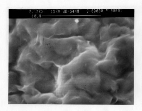
Fig. 4. SEM image of 1  $\mu$ l SWy-1 spin-coated film viewing from the back side of the film.
