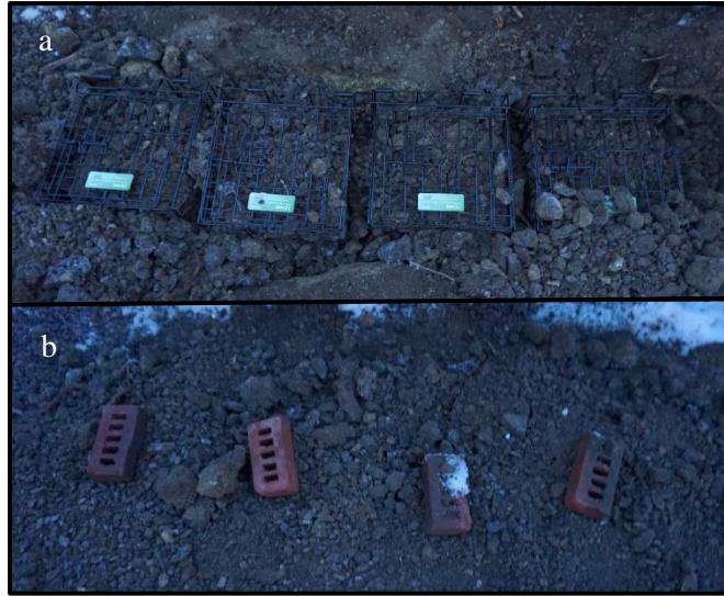
Figure 15. Buried cages completely covered: a) cages filled with specimens and soil; b) bricks signifying the placement of each cage.
