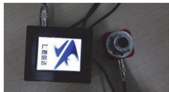
Figure 11. Crack width measuring instrument
