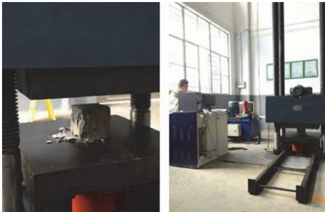
Figure 2. Test block compression test
