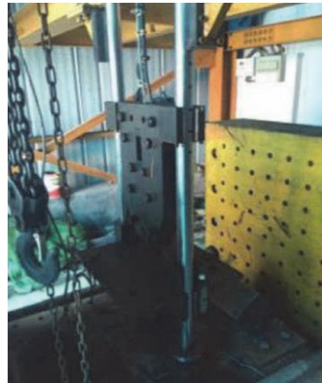
Figure 5. Drop hammer test machine
