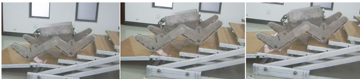
Fig. 16 Stairs-climbing test on the test platform
