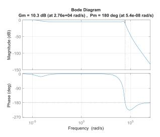
Figure 9b. Bode plot of the resulting multiple section input filter
