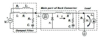
Figure 6a. Series damped filter
