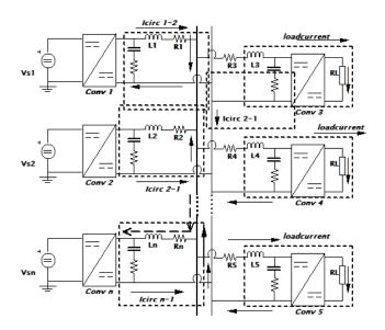
Figure 3. Circulating current problem among a multi-converter system
