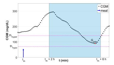
**Figure 1.** Graphical representation of the classification scheme. Black dots are the continuous glucose monitoring (CGM) samples. Blue stem indicates the meal event. Red dot is the minimum glucose level  $G_{\min}$  reached in the fixed postprandial window ( $t_m + 2 h$ ,  $t_m + 6 h$ ; highlighted in light blue). Horizontal magenta lines denote the thresholds used to discretize  $G_{\min}$  into the classification target Y.
