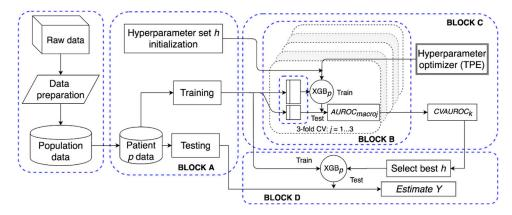
**Figure 2.** Structure of the proposed extreme gradient-boosted tree  $(XGB_p)$  software framework. After data preparation, for patient p, block A initializes h and splits the data in training and test; block B computes the performance of the hyperparameter set in a three-fold cross validation (CV) setting over the training set; block C implements a tree-structured Parzen estimator to optimize h; block D selects the best h set and evaluates the performance of  $XGB_p$  on the test set.
