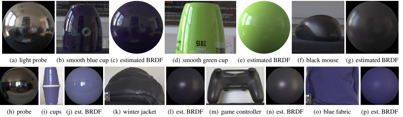
Figure 8: Additional results of example-based material appearance estimation in indoor lighting environments. Top-row: BRDFs estimated in an office environment for two coffee cups with smooth surfaces and a rough specular black plastic mouse . Second-row: BRDFs estimated in a living room environment for a blue plastic cup , a winter jacket , a game controller , and blue apparel fabric .
