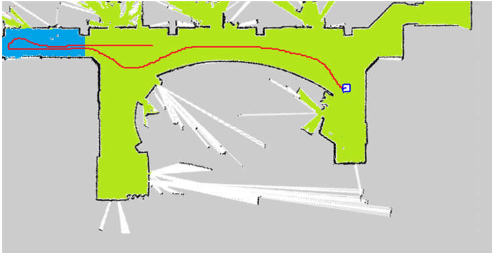
Figure 4.11 – Map of the robot's trajectory on the floor; green colour indicates carpet and blue indicates plastic surface
