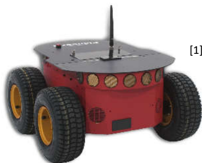
Figure 2.4 – The Pioneer 3-AT robot platform; used in different research on outdoor surface classification
