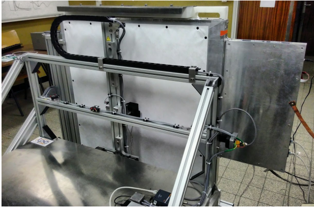
Fig. 5. The Calipso quality assurance setup, which used a full scale prototype SoLid electronics enclosure. The enclosure, dubbed ‘Zoidberg’, read out over 100 million neutrons during the QA campaign to ensure a uniform plane response.
