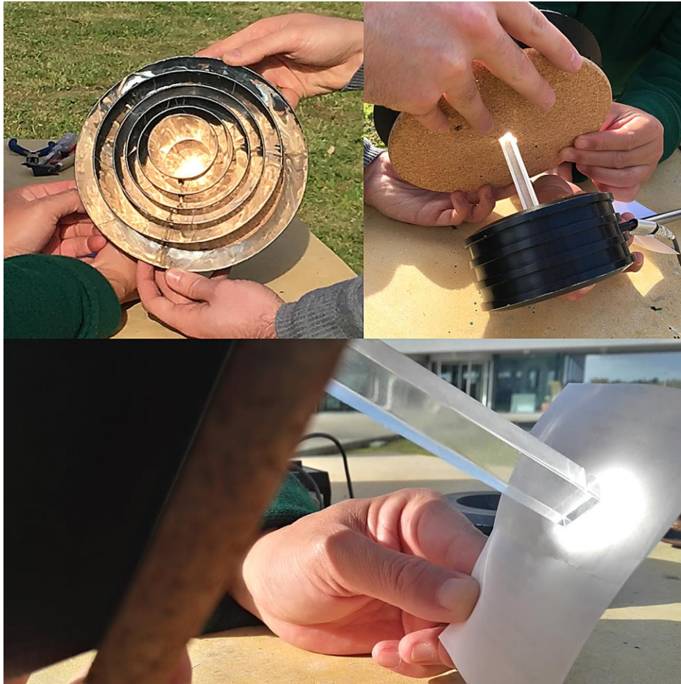
Figure 8.1 - Ring-array 1:7 scale model first prototype ring displacement and focusing adjustments.
