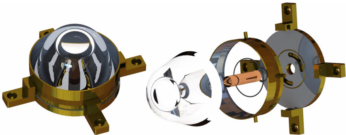
Figure 8.7 - SOLIDWORKS™ rendered view of the assembled and exploded rendered views of the laser head, showing the aspheric fused silica, the 5.0 mm diameter and 20 mm length Nd:YAG rod, the silvery-coated pump cavity, two O-rings, and the base with the cooling channels.
