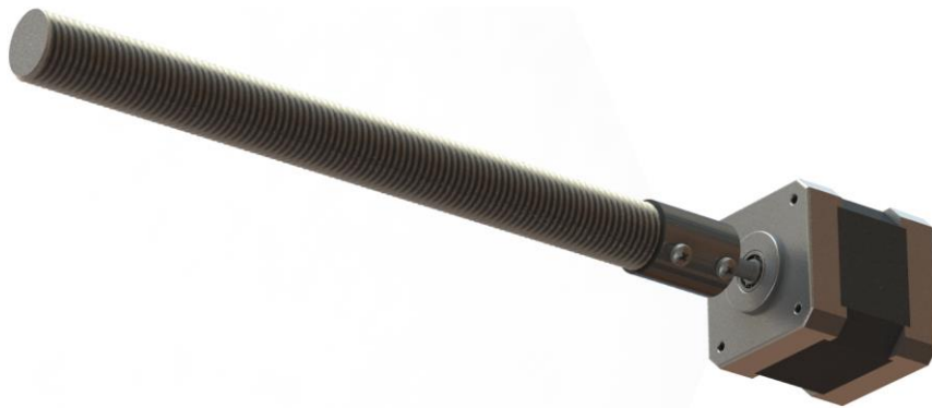
Figure 8.11 - SOLIDWORKS™ Rendered view of the 162 mm M16 threaded rod, the stepper and the link between them.
