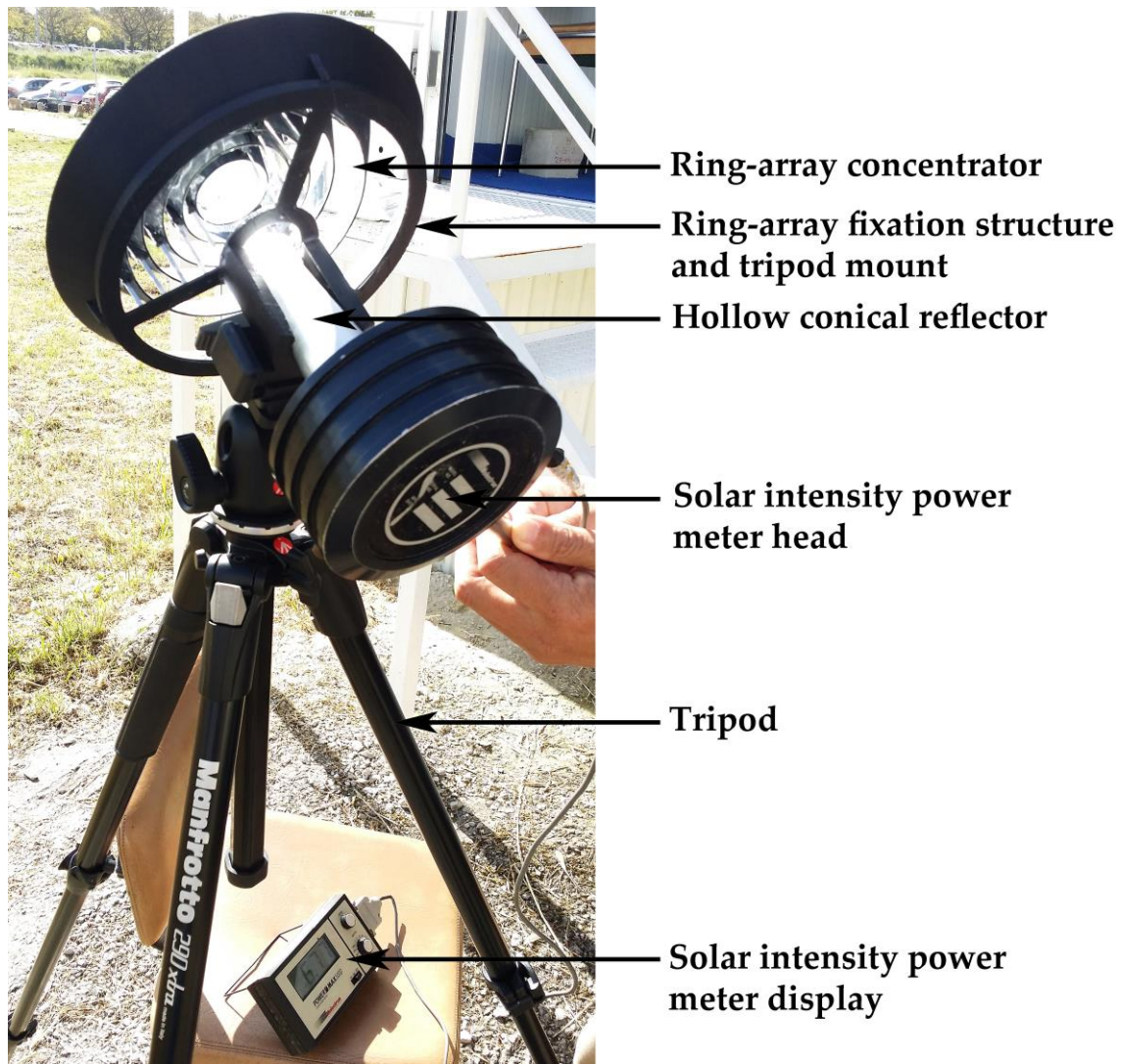
Figure 8.6 – Concentration solar power testing with the 1:7 scale model assembly in a tripod mount specially designed and settled for this purpose.
