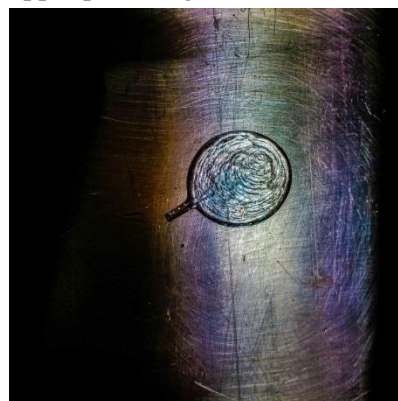
Fig. 10 The glass sample quenched between two copper plates.
