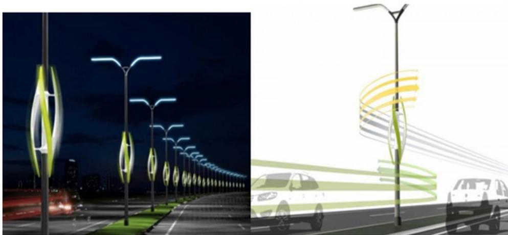
Figura 1. 10 Wind - turbine powered highway lights, conceito de TAK Studio adaptado de [17].
