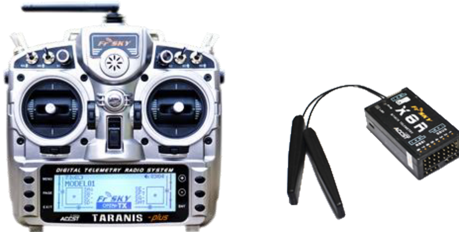
Figure 3.6: FrSky Taranis X9D Plus on the left and its receiver on the right.
