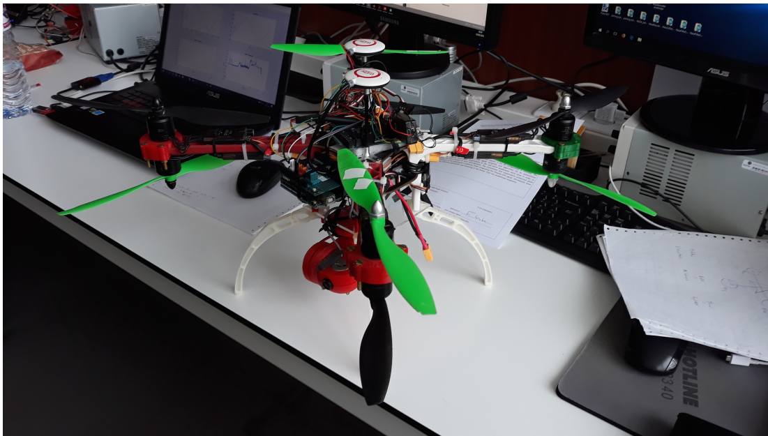
Figure 5.10: X8-VB Quadcopter featuring two GPS sensors for improved localization data.
