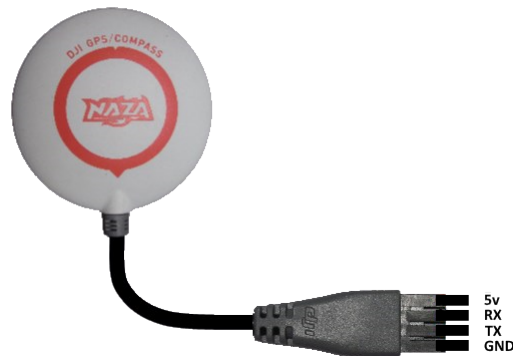
Figure 3.11: NAZA GPS wiring.
