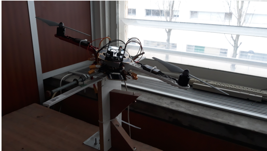
Figure 5.11: Test bench for the NAZA controller identification.
