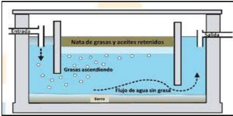
Figura 7. Trampas de Grasas, Clean water Technology 51
