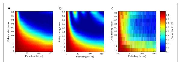
**Figure 3.** Transfer efficiency for different delay scaling factors and pulse length for blue sideband transitions for a ground state cooled ion. (a) Simulation using the three level approximation and (b) the full Hamiltonian as well as (c) experimental data for the STIRAP transfer. Red corresponds to no and blue to complete transfer.
