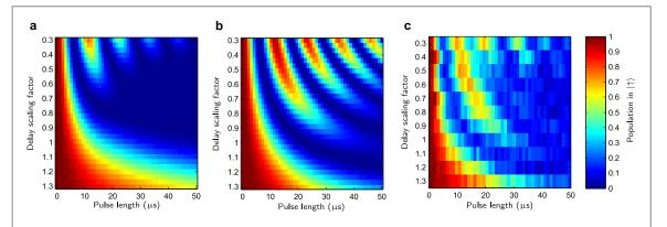
**Figure 2.** Transfer efficiency for different delay scaling factors and pulse length for carrier transitions for a ground state cooled ion. (a) Simulation using the three level approximation and (b) the full Hamiltonian as well as (c) experimental data for the STIRAP transfer. Red corresponds to no and blue to complete transfer.
