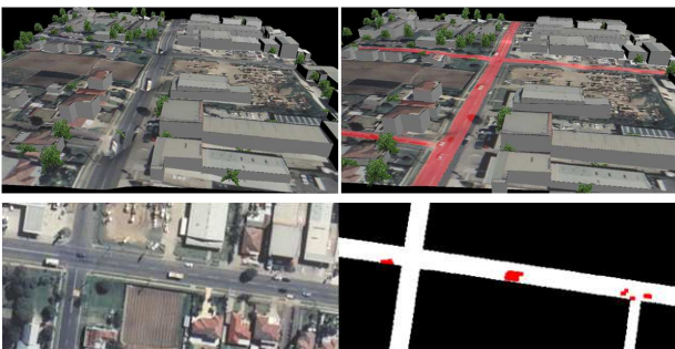
Figure 6: Top left: part of the model view for the data-set Fairfield ; model was generated from the depth map of Fig. 3, right. Outliers caused by moving object are clearly visible. Right: similar view of the improved model; pixel belonging to street have been identified by means of GIS data and are marked in pink. Bottom left and right: Deviations between the original and the corrected DSM provide alarms about moving objects. After applying some morphological operations, several moving vehicles have been detected.
