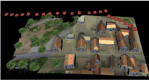
Figure 9: A view of the textured model from the data set Bonnland . Camera positions corresponding to the reference images are depicted by red viewing cones while the image on the left of Fig. 2 is used to texture the terrain and building roofs. A typical facade for the region is used to texture building walls. The trees are modeled in the elevated tree-like pixel areas of Fig. 2.
