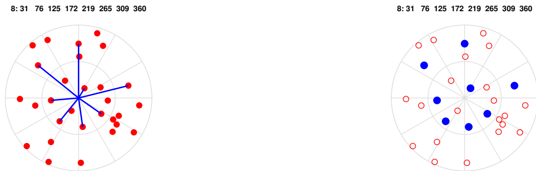
Figure 5: The set of m = 8 star best fitting Bowditch's sense of spread; the HDOP equals 0.7079.
