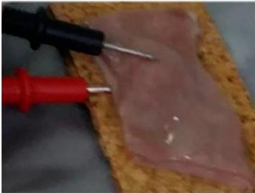
Figure 1 Evaluation of electrical resistivity with a multimeter.
