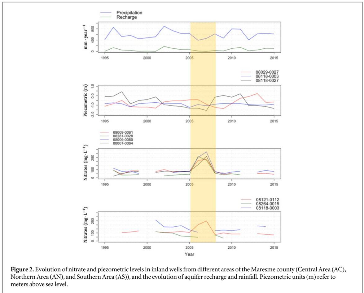
**Figure 2.** Evolution of nitrate and piezometric levels in inland wells from different areas of the Maresme county (Central Area (AC), Northern Area (AN), and Southern Area (AS)), and the evolution of aquifer recharge and rainfall. Piezometric units (m) refer to meters above sea level.
