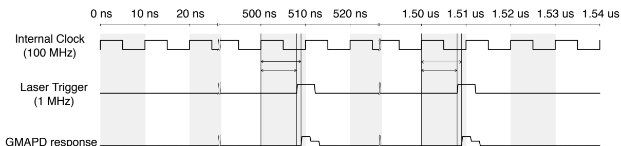
FIGURE 2.10: The phase shift between the laser’s pulse and a detected photon can be obtained by subtracting the laser pulse’s timestamp from the timestamp of the detected photon. This subtraction has to occur between timestamps acquired within a period of f^{-1} , where f is the laser’s pulse repetition frequency.
