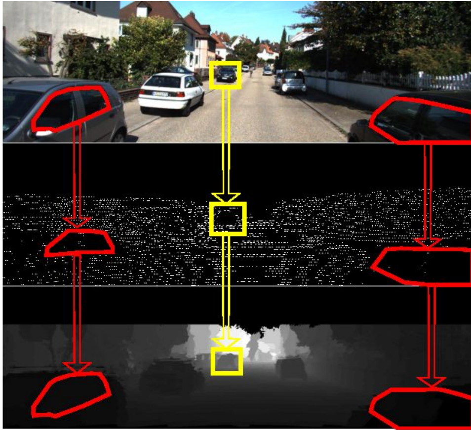
Figure 2.8. Top: RGB scene. Middle: sparse depth image. Bottom: dense depth image [28]
