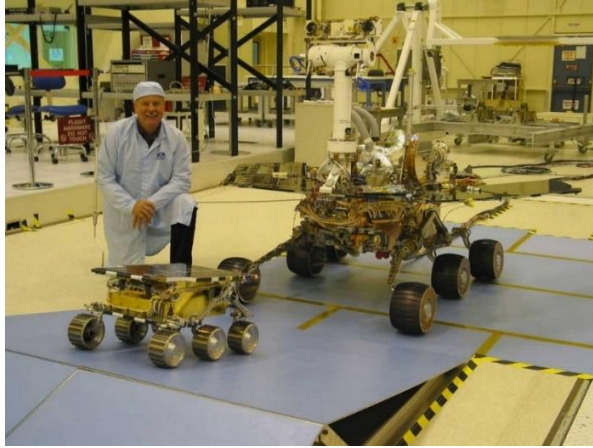
Image 3: Mars Exploration Rover (rear) vs. Sojourner rover (Courtesy NASA/JPL-Caltech/Wikipedia).
