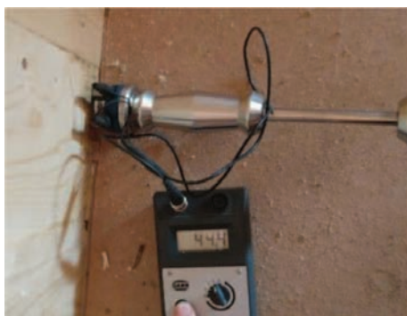
Figure 2.1. MC measurement device (a), external wall section with sensors placement (b).
