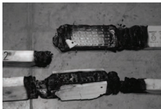
Figure 2. Failure characteristics of unprotected joint (a) and gypsum plasterboard encapsulated joint (b).
