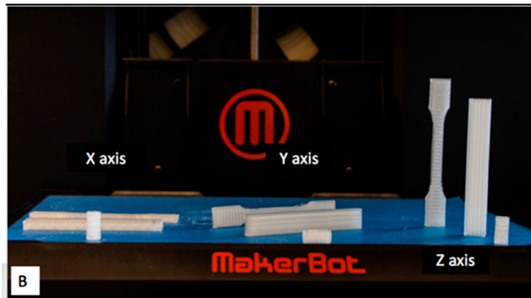
Figure 1. 3D Printed poly(lactic acid) (PLA) constructs (compression cylinders, flexural bars and dog-bone shape) in different orientations.
