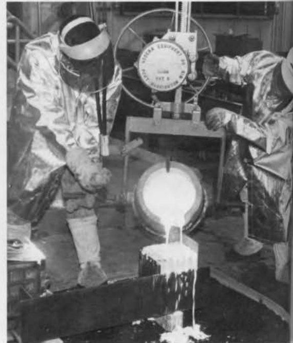
Using brass, junior Mike Formanek and sophomore Greg Quick pour the molten liquid into molds. Later, the brass is removed producing a sign or plaque. • Shelley Mugge
