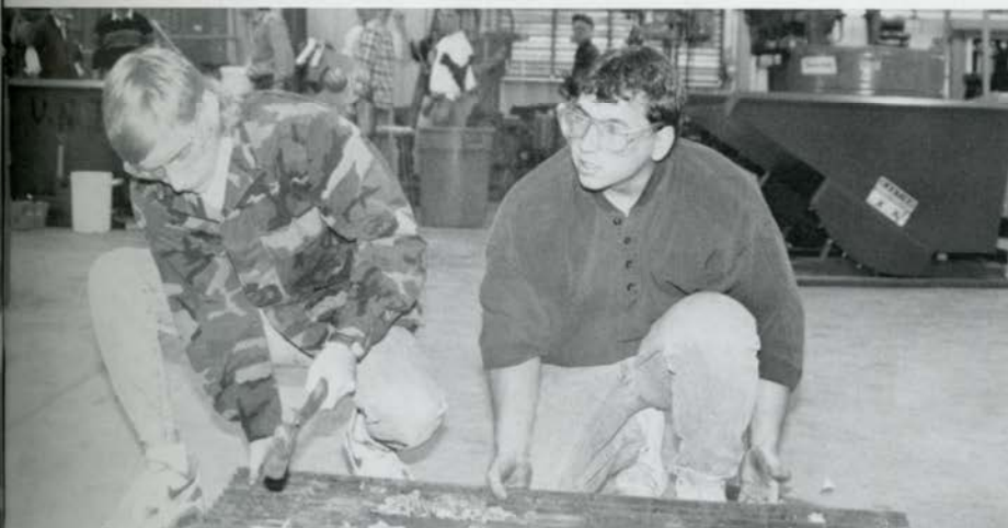
Freshmen Weylon Heiser and Kevin Bock work on the floor of the center to hammer hardened metal off of a grid. The metal they chip off was melted down to be used again.
