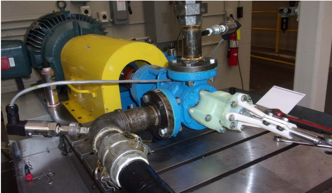
Figure 25: Test Setup Discharge Port at 90°
