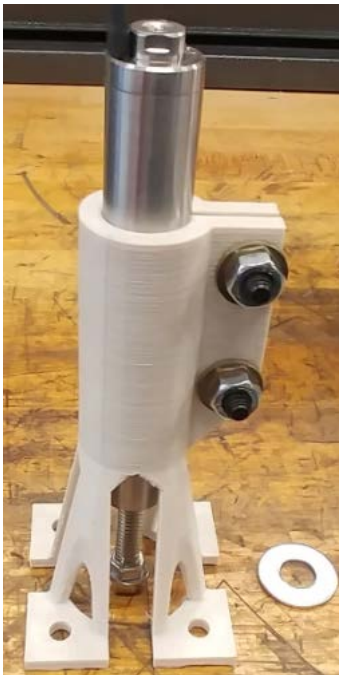
Figure 24: LVDT Sensor with FDM 3D Printed Mounting Bracket
