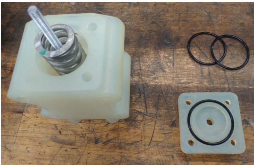
Figure 20: Assembly of Prototype Valves
