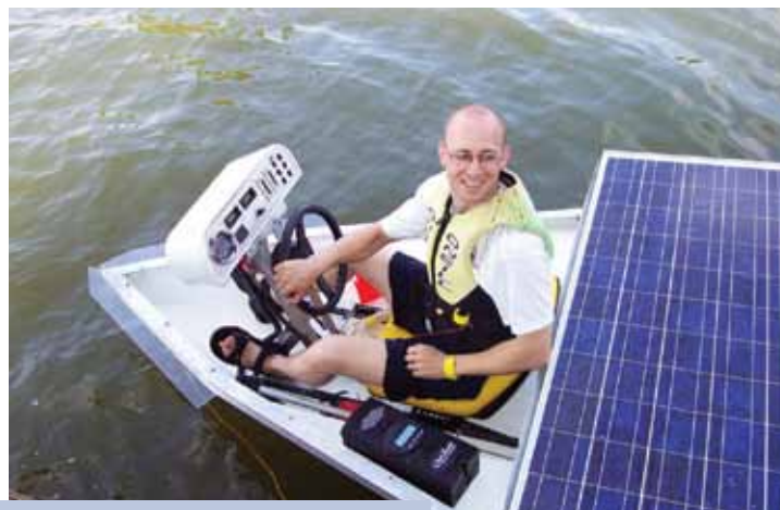
Team leader Mike Boomer waits for the final call to begin the race after completing safety inspections at the Solar Splash. The black box is a solar panel/battery charge controller to monitor voltage, current and temperature in the deep cycle battery bank.
