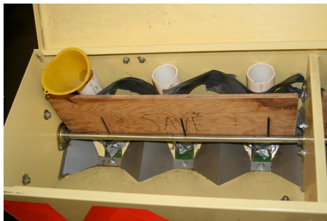
Figure 3. Seed drill modification for planting small areas
