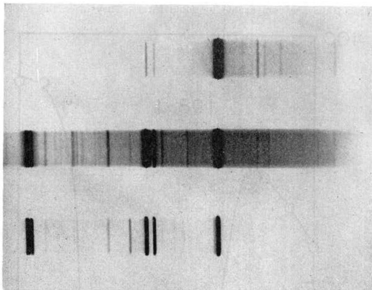
Figure 6. Raman spectra of benzene. (Simultaneous exposures). Top—tube coated with acetate and Rhodamine—Beetle filters. Middle—no filter. Raman lines excited by both 4047 A and 4358 A may be seen, partially obscured by the continuous background. Bottom—mercury spectrum.
