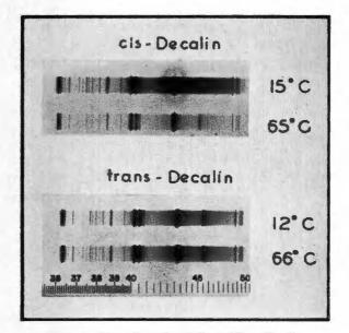
Figure 1. Raman Scattering of Cis- and Trans-Decalin.
